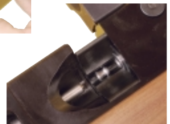
Below: Shows the single shot holder in place ready to load in pellet.
