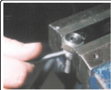
View showing the main seal tightening procedure for the metal valve using the collet and rod supplied with service kit.
